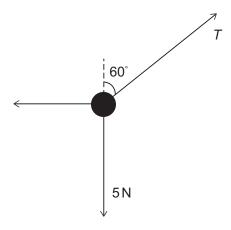
*T* is the tension in the diagonal rope.
