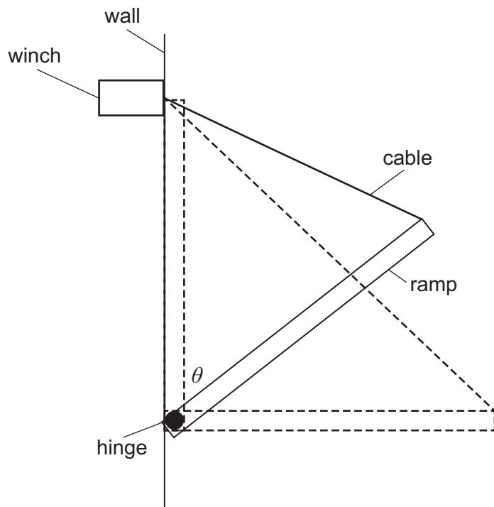
The ramp is lowered slowly, at constant speed, from its closed (vertical) position ( $\theta = 0^\circ$ ) to its open (horizontal) position ( $\theta = 90^\circ$ ).
