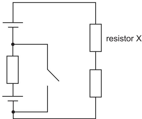
What is the power dissipated by resistor X after the switch is closed?
