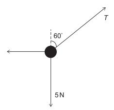
*T* is the tension in the diagonal rope.
