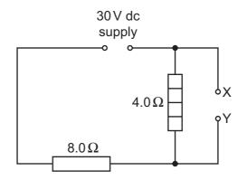
The power transferred in the 4.0  $\Omega$  heater is 9.0 W.
