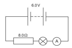
The reading on the ammeter is 0.25 A.
