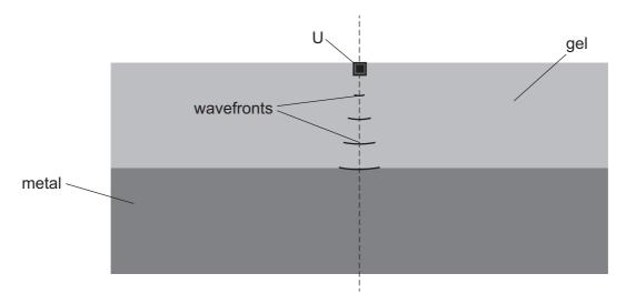
Ultrasound travels faster in the metal than in the gel.
