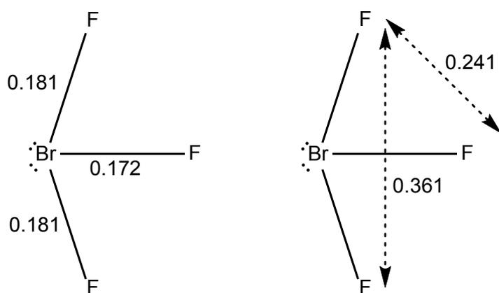
Finding a right-angled triangle using appropriate distances, and using the inverse sine function ( $\sin^{-1}$ ), gives the bond angle as  $\sin^{-1}\left(\frac{0.1805}{0.181}\right)$  ( $= 86^\circ$ )
