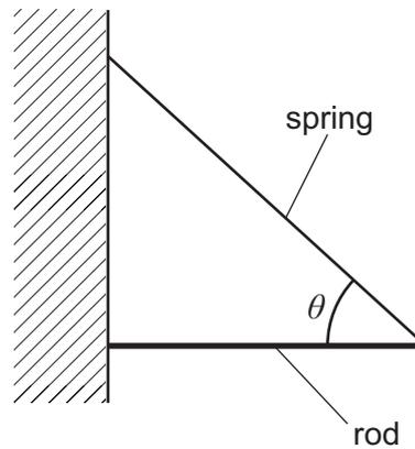
The spring constant of the spring is  $20 \text{ N m}^{-1}$  and the weight of the rod is  $16 \text{ N}$ .
