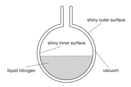
The vessel has a double wall made from a poor thermal conductor. There is a vacuum in the gap between the two walls.
