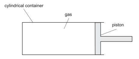
The particles of the gas are moving with an average speed v, and collide with the surface of the piston with a frequency *f*.
