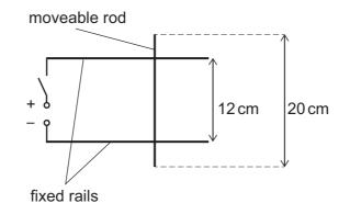
The whole arrangement is placed in a uniform magnetic field of magnitude 0.50 T that is directed perpendicularly into the page.
