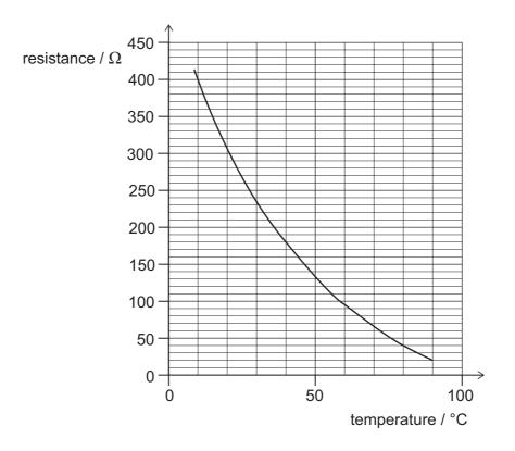
When the temperature of the thermistor is  $10 \degree$ C the current in the circuit is 25 mA. What is the current when the temperature of the thermistor is  $80 \degree$ C?
