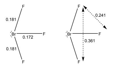
Finding a right-angled triangle using appropriate distances, and using the inverse sine function  $(\sin^{-1})$ , gives the bond angle as  $\sin^{-1}\left(\frac{0.1805}{0.181}\right)$  (= 86°)
